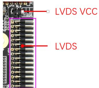
General LVDS interface definition, support single / dual, 6/8 / 10-bit 1080P LVDS screen. The screen voltage can be selected through a jumper cap, and it can be selected to support 3.3V / 5V / 12V screen power supply. In order to avoid burning boards and screens, please note the following:
