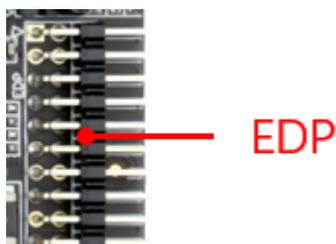
This interface is a common EDP screen interface in the form of 10\*2 double-row pins. The screen voltage can be selected through the jumper cap, and it can choose to support 3.3V/5V/12V screen power supply.
