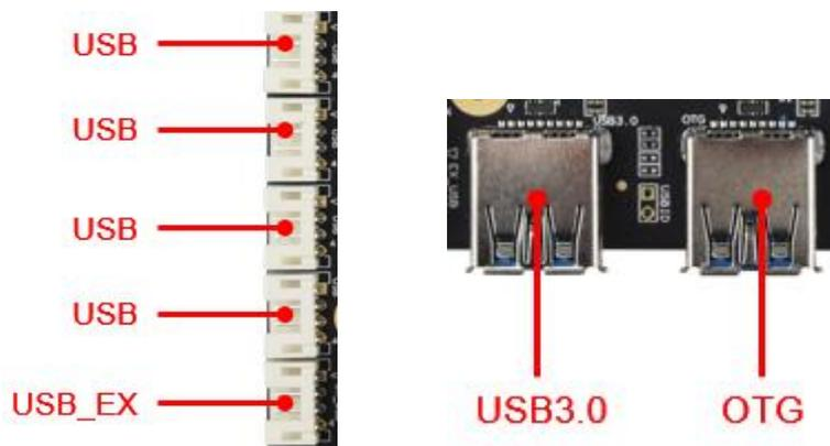
The board has 2 USB standard interfaces and 4 USB pins, one of which is shared with the 4G module.
