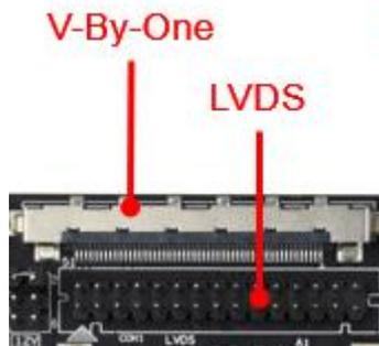
General LVDS interface definition, support single/dual, 6/8/10 bit 1080P LVDS screen. The screen voltage can be selected through the jumper cap, and can choose to support 3.3V/5V/12V screen power supply.
