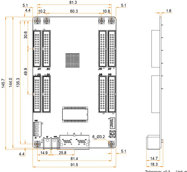
Tolerance: ±0.3 Unit: mm
