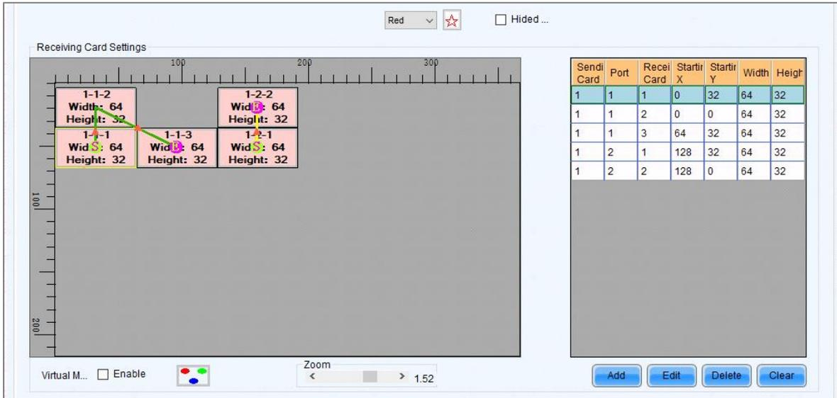
Step 8 Click **Send to HW** to send the configuration information to the hardware. If necessary, click **Save to File** to save the configuration information as a file.
