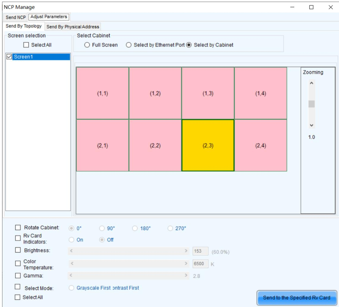
Step 9 Click **Send to Specified Rv Card** once you are done to send the firmware program and configurations to the receiving cards.
