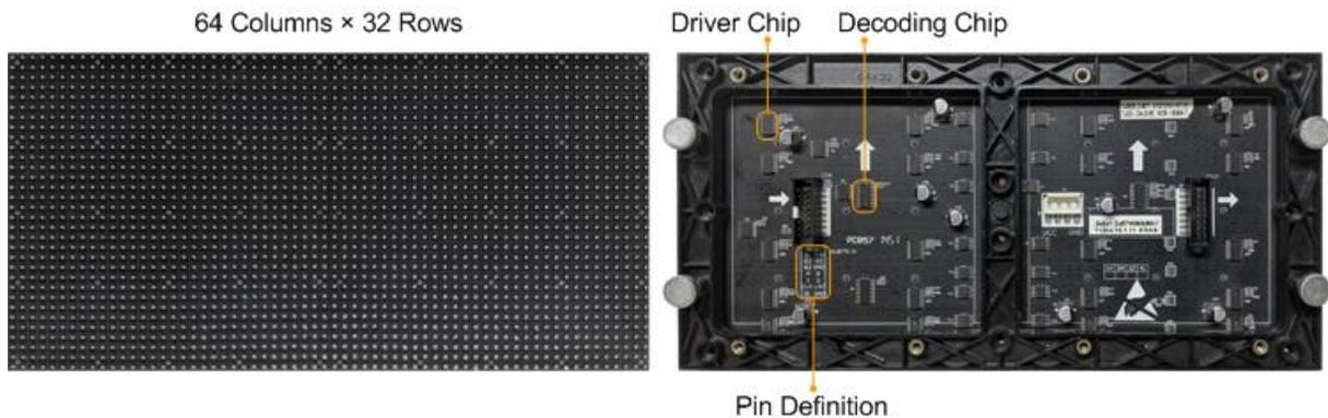
Both regular and irregular modules are rectangular. If the module column quantity can be divided by 16 without remainder, the module is a regular one.
