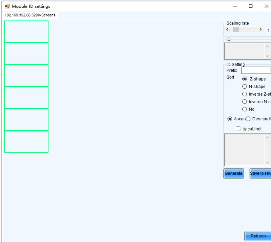
Step 5 Select the ID generation method. Click **Generate** to set IDs for all the modules, or double click a single module and set its ID in the displayed dialog box, and then click **OK**.
