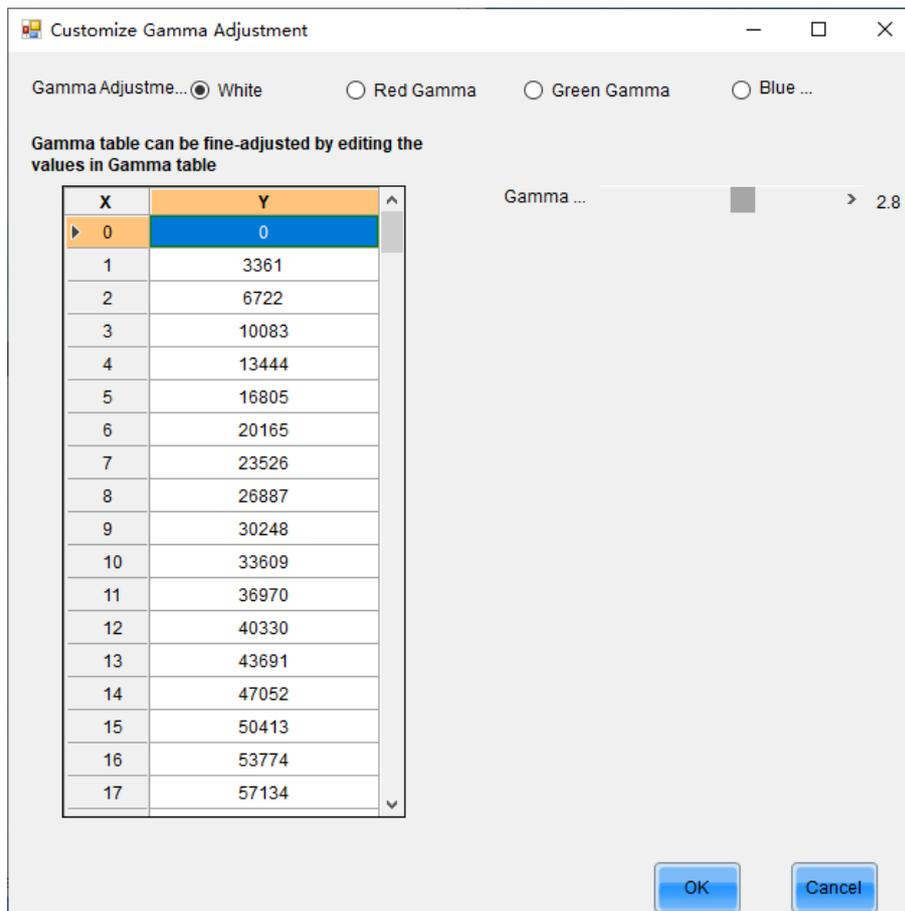
Step 3 If the control system supports individual Gamma adjustment for RGB, select **White** to adjust the Gamma curves for red, green and blue at the same time. Or, select **Red Gamma**, **Green Gamma**, or **Blue Gamma** to adjust the Gamma curve for a single color. If the control system does not support individual Gamma adjustment for RGB, skip this step.
