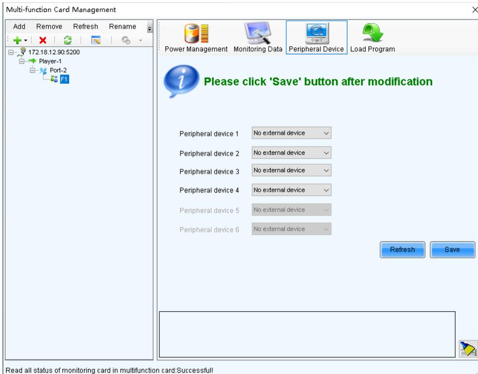
Add peripheral devices connected to the multifunction card, including the light sensors and external 3D emitters.
