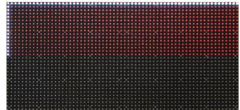
Step 13 View the flashing pixel in the first column on the module and click the corresponding cell in the grid to draw the pixel position (You can also use the keyboard arrow key to quickly draw the position), and click **OK** after the drawing is done.
