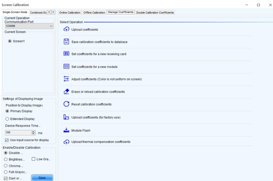
Step 6 Perform the following operations as required. During the operation, you can select **Disable Calibration**, **Brightness Calibration**, **Chroma Calibration**, or **Full-grayscale Calibration** on the left. **Dark or Bright Line Correction** and **Low-grayscale Calibration** can be selected at the same time. After saving, you can view the effect of applied coefficients on the screen.
