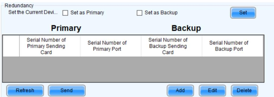
**+** Configure device redundancy
