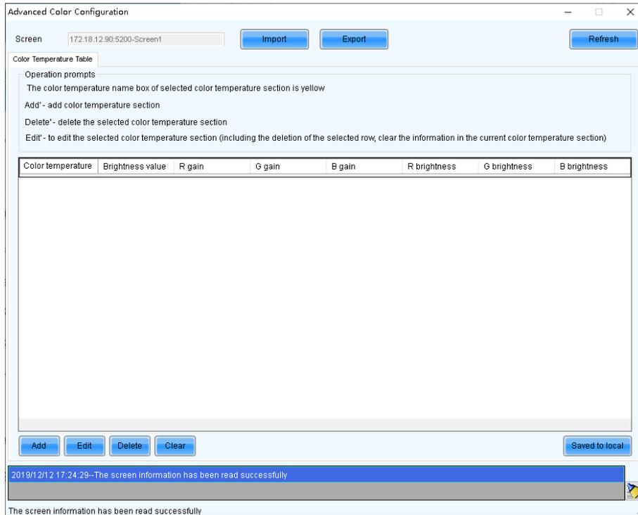
Step 3 If you have a color temperature configuration file (.fcg), click **Import** to complete the configuration quickly. If you do not have a color temperature configuration file, continue performing the following operations to manually complete the configuration.
