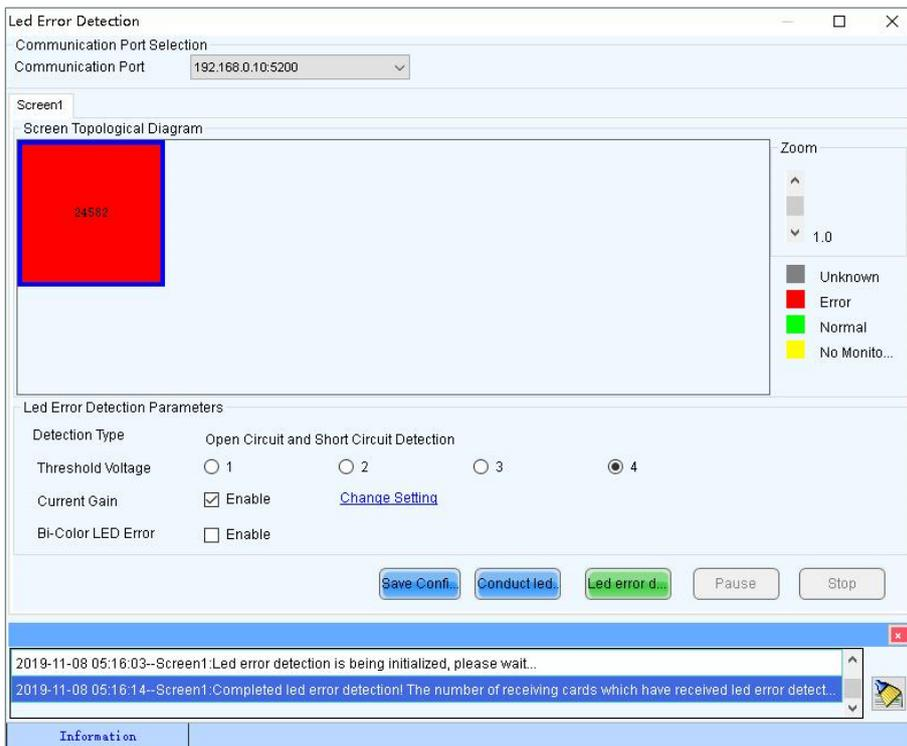
The number displayed on the topological diagram indicates the number of the faulty LED lights. Hover the mouse over the topological diagram to view the detailed Led error detection information.
