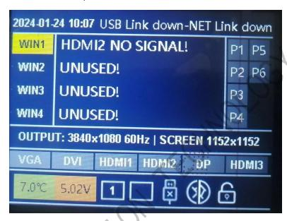
It accurately displays the signal source resolution, each window information, network port connection status, key lock status, USB debugging cable connection status and other information input from our front end.
