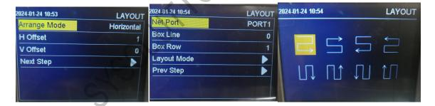
Arrangement mode, select horizontal and vertical arrangement, set horizontal and vertical offset, next step, set the number of cabinet columns, cabinet rows, wiring method, and set the next network port after completion.
