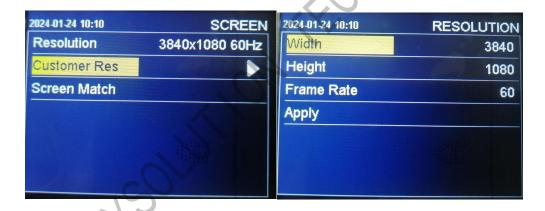
When there is no output resolution that meets our needs among the 18 preset output resolutions, such as 1920X1280 size, then it is necessary to customize the resolution. Specific operations: Main menu - "Output Display" - "Resolution" - " Custom Resolution", set the screen width to 1920, the screen height to 1280, the refresh rate to 60, and apply.
